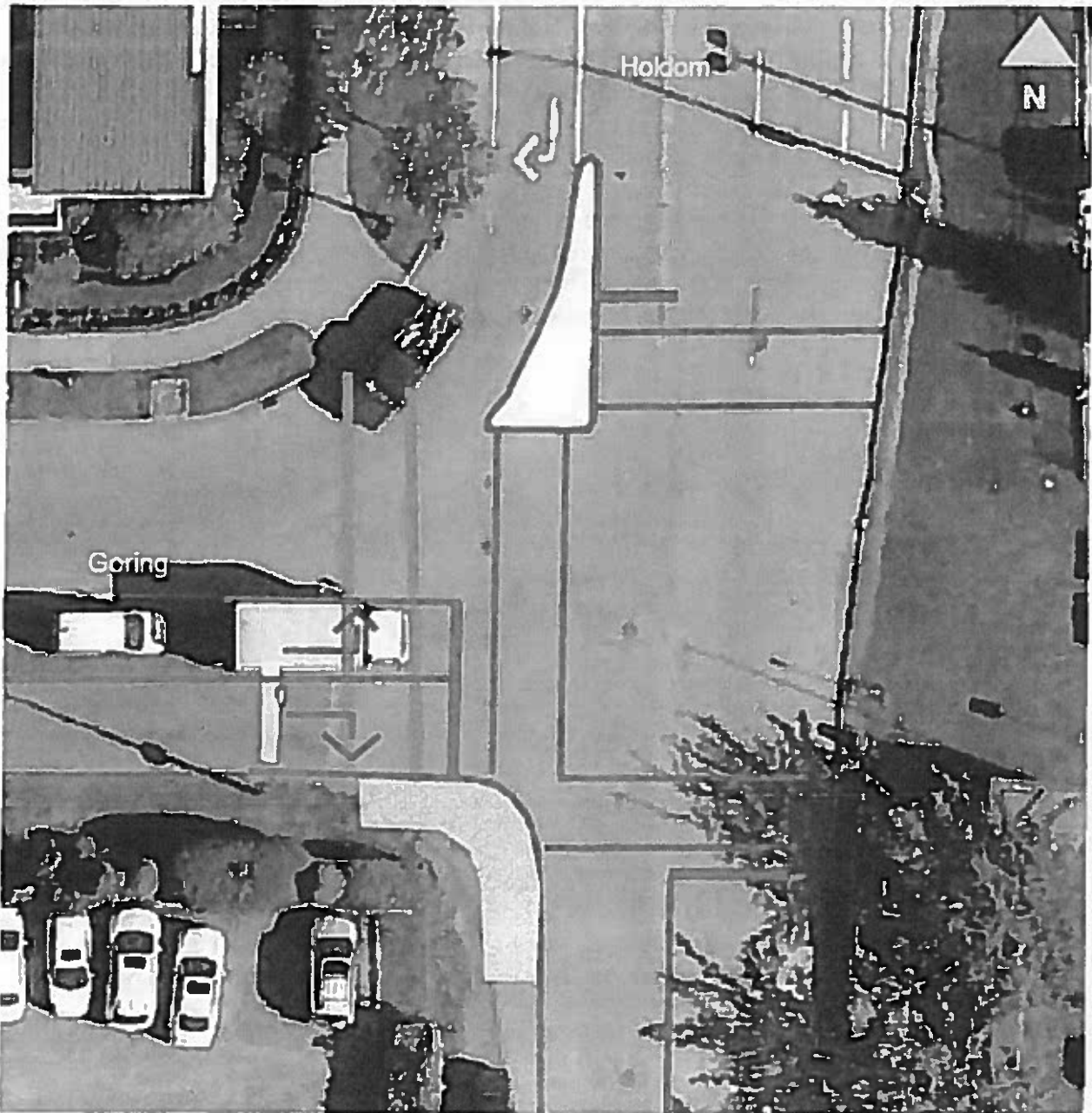
Figure 2: Recommended Traffic Control Upgrades at the Goring/Holdom Intersection
