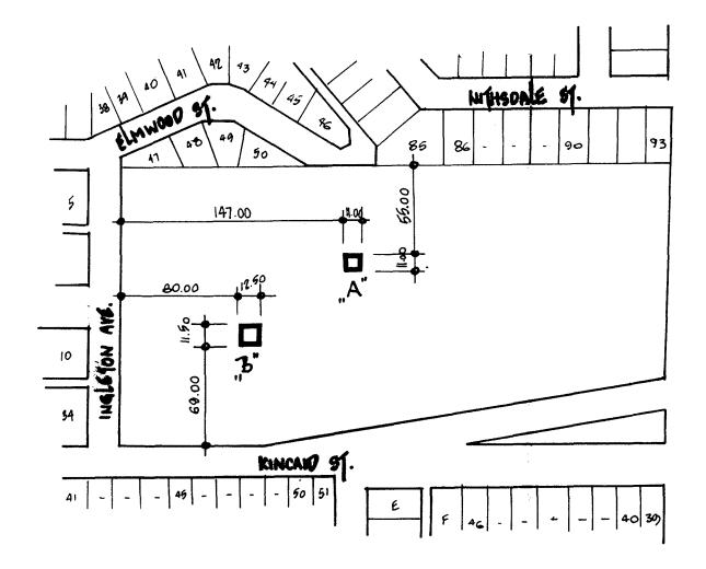
"A" - P2 DISTRICT ZONING WITHIN AN AREA 11M X 11M ABOVE GEODETIC ELEVATION 108.09 METERS
