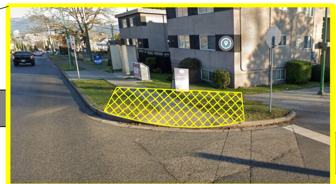
Yellow hatched area depicts flagger location and escape route.
