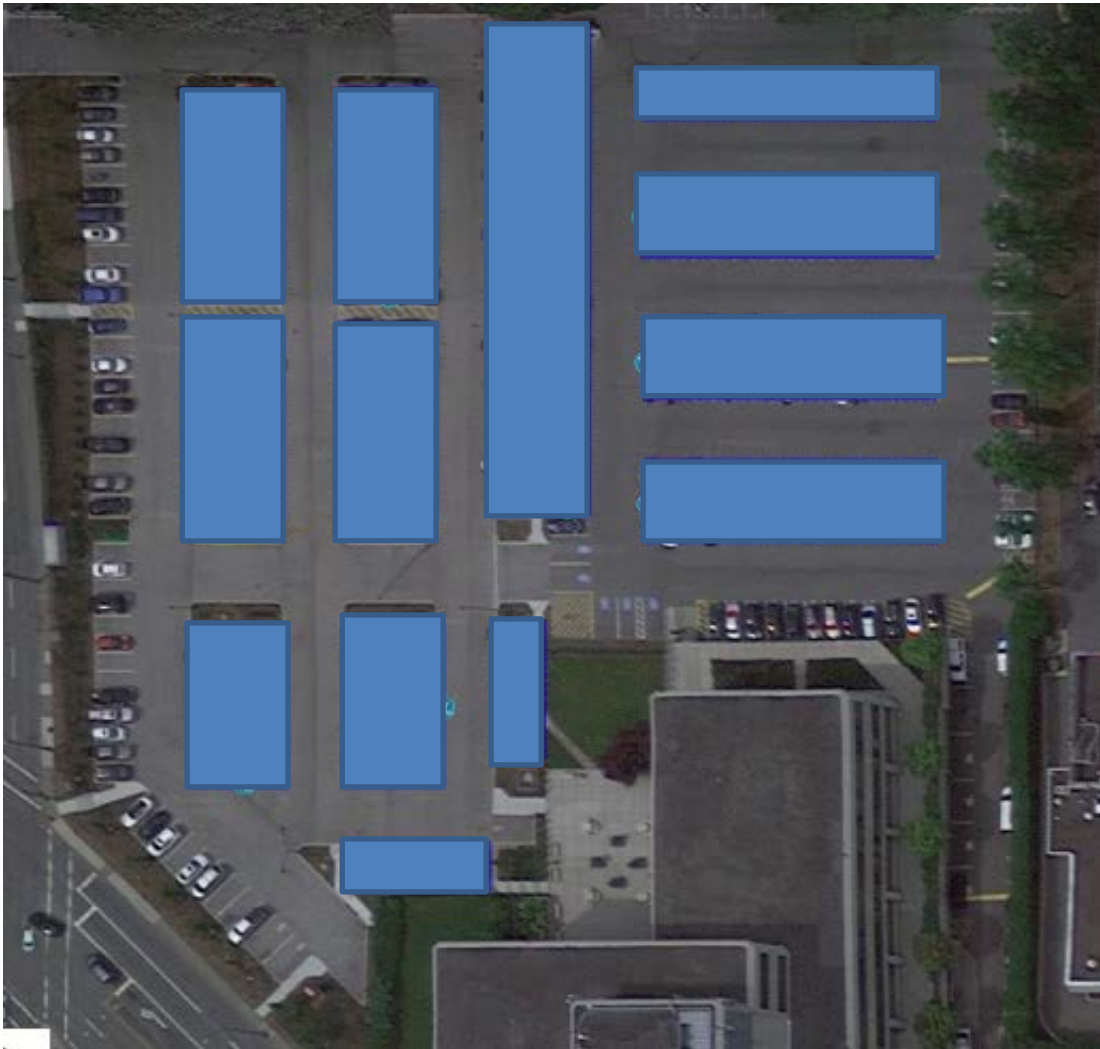
Ground Mounted PV Solar Parking Canopy Canada Way/Norland
